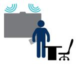
Presence sensor will detect the person entering the room and the display will turn on
